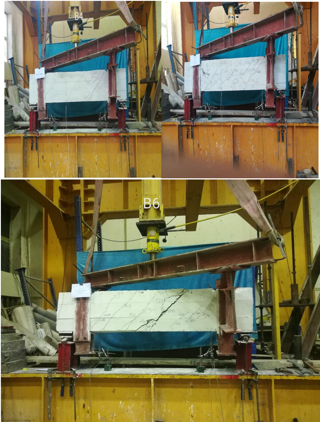
Figure (13): Tested beams at failure: B4, B5 and B6
