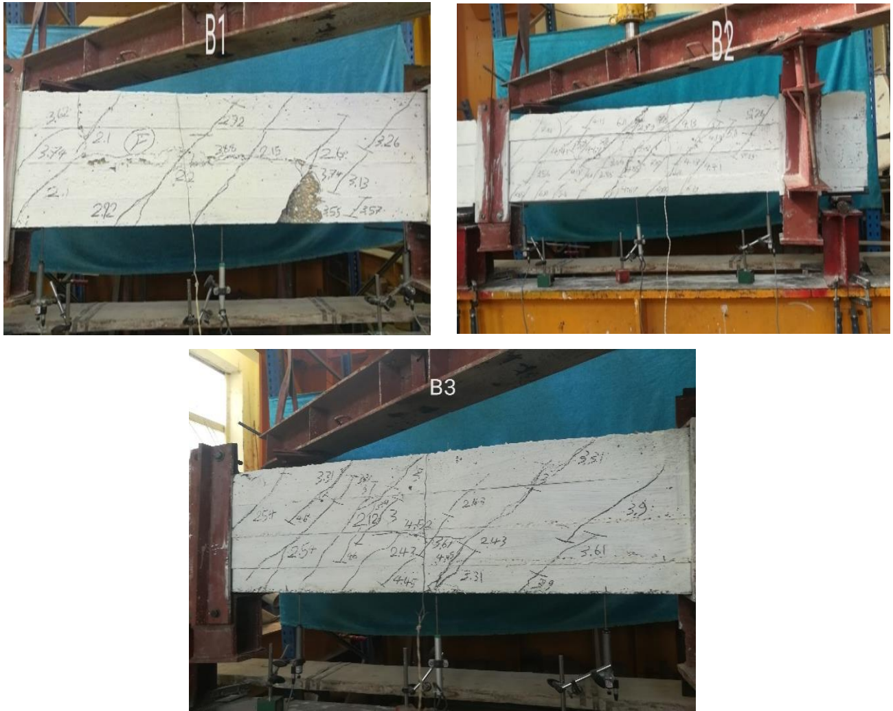
Figure (11): Tested beams at failure: B1, B2 and B3
